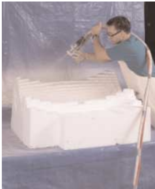
Spray RAYITE 200 on undersized armature.
