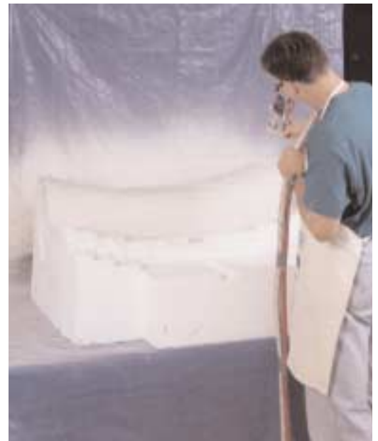
Spray RAYITE 200 to slightly oversized tolerance.
